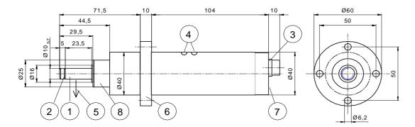
1 = Shaft5 = Loading direction 2 = Seegerring A10 6 = Mounting flange
