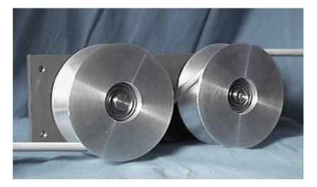
The tensile - force measuring - station 2 R 80 is a space-saving solution for precise measurement of cables, wires, tirecord and other flexible material.
