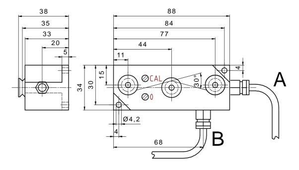
Sensor series LC 1321 is equiped with built-in amplifier. It supplies an outputsignal of 0 up to +10 V, corresponding 0 up to 100% the nominal load. To adjust the electrical zero and the gain ( calibration ), corresp. potentiometer are accessible at the front page.
