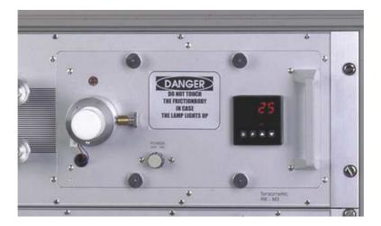
The measuring unit of the Frictionmeter RK-M3 can be equipped with a friction body heating system.
