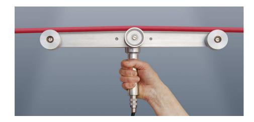
Head series M 150 is a compact system to measure tensile forces on: cables, belts, profiles, tapes etc. The smooth, in precise ball-bearing running rollers, can be adjusted to the material, which should be measured.
